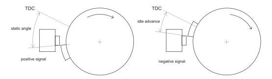
When "only [+] signal" is selected, then only positive signal is detected and ignition timing is calculated for all revs as programmed with ignition map.
