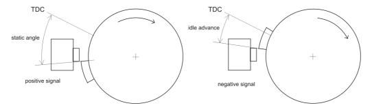
When "only [+] signal" is selected, then only positive signal is detected and ignition timing is calculated for all revs as programmed with ignition map.
