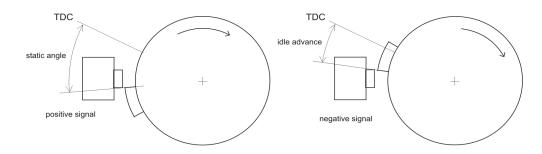
When *Trigger Mode 1* is selected, then only positive signal is detected and ignition timing is calculated for all revs as programmed with ignition map.
