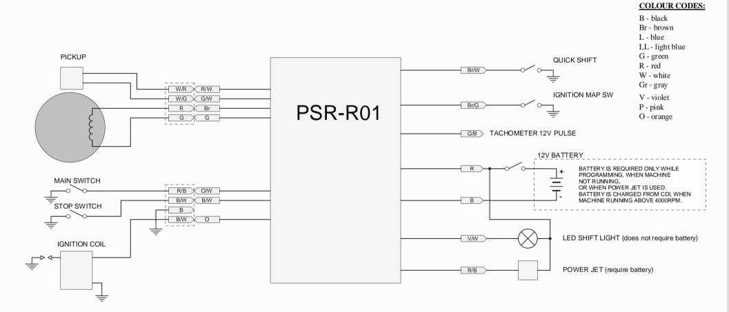
PSR-R01 IS PROGRAMMABLE CDI AND RUNS WITHOUT BATTERY IT CAN BE PROGRAMMED WITH HANDHELD PROGRAMMER AND PC
