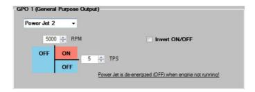
Power Jet 2 change state when revs and TPS are higher/lower then programmed value.
