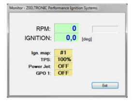
⇒ Monitor show engine revolution, ignition advance angle, TPS position, selected ignition map, rev limit operation, power jet operation, GPO operation.
