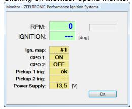
⇒ Monitor shows engine revolution, ignition advance angle, selected ignition map, rev limit activation, GPO output state, pickup signal test and power supply voltage.
