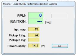
⇒ Monitor shows engine revolution, ignition advance angle, selected ignition map, rev limit activation, pickup signal test and power supply voltage.
