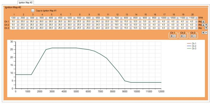
Each ignition output channel can be programmed with separate ignition curve.
