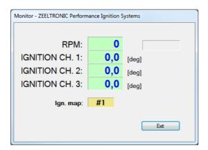
⇒ Monitor shows engine revolution, ignition advance angle, selected ignition map, rev limit.
