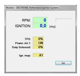
⇒ Monitor show engine revolution, ignition advance angle, TPS position, selected ignition map, rev limit operation, power jet 1 operation, duty solenoid operation
