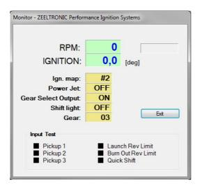
⇒ Monitor show engine revolution, ignition advance angle, selected ignition map, shift light operation, rev limit operation, power jet operation.
