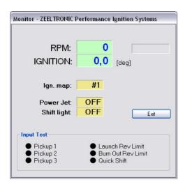
⇒ Monitor show engine revolution, ignition advance angle, selected ignition map, shift light operation, rev limit operation, power jet operation.
