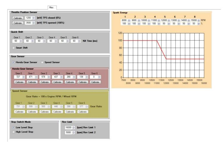
⇒ Calibrate TPS Close Position ... click on 'Calibrate' button beside TPS closed position value and new window will open. Hold throttle at full close position and click 'OK' to confirm new calibration, or click 'Cancel' to abandon calibration.
