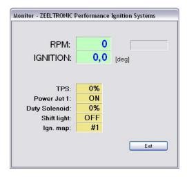
➡ Monitor show engine revolution, ignition advance angle, TPS position, selected ignition map, shift light operation, rev limit operation, power jet 1 operation, duty solenoid operation
