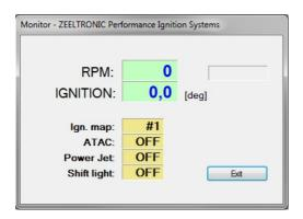
⇒ Monitor show engine revolution, ignition advance angle, selected ignition map, shift light operation, rev limit operation, power jet operation.
