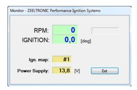
⇒ Monitor show engine revolution, ignition advance angle, selected ignition map, rev limit activation and power supply voltage.
