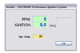
⇒ Monitor show engine revolution, ignition advance angle, selected ignition map and rev limit activation.
