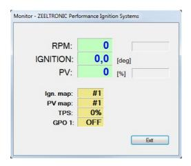
⇒ Monitor shows engine revolution, ignition advance angle, PV position, TPS position, selected ignition and PV map, rev limit operation, GPO operation.
