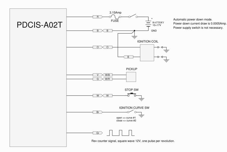
CDI have to be placed inside sealed e-box to prevent flooding and possible damage of CDI unit.
