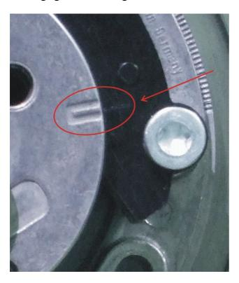
Ignition timing needs to be set to 23deg, when marks on the rotor and stator are aligned. Set ignition timing with dial gauge, or timing wheel.
