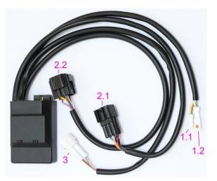
Connector **3** is for the switch/ push button used to select the operation mode. To keep the servo permanently in the open position (without using a switch/ push button), connect the **brown** and **brown/white** wires together at the connector **3**.
