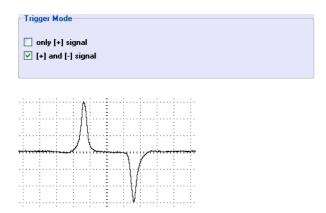
Trigger signal from pickup consist of positive and negative pulse. Positive pulse must be first and is generated by leading edge of trigger bar...negative pulse must be second and is generated by trailing edge of trigger bar.
