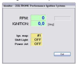
⇒ Monitor show engine revolution, ignition advance angle, throttle position, power jet, selected ignition map and rev limit activation.
